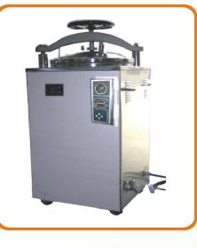
Sterilizing record: Micro-printer (recording the whole process) diagnosing & alarm system Water supply system: Reservoirs (3.5L fresh water & 5L waste water)
